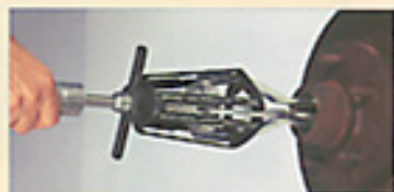
Bearing cup removal from brake rotor
