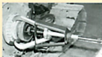
Drive sprocket removal (Model 116)
