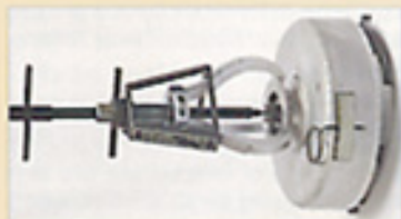
Washing machine clutch removal (Model 103)
