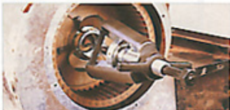
Blower wheel removal made easy (Model HP-2)
