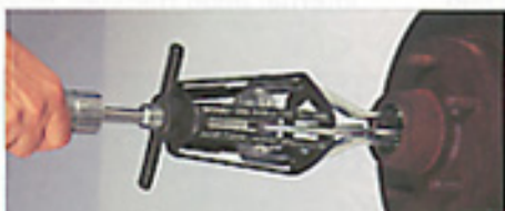
Bearing cup removal from brake rotor (Model 105)
