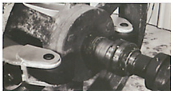
Clamping jaws on inside of pulley hub
