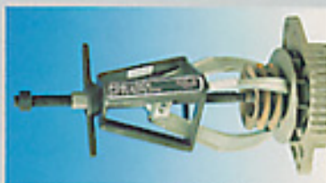
Alternator pulley removal (Model 106)
