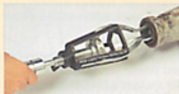
Oil seal removal from transmission housing
