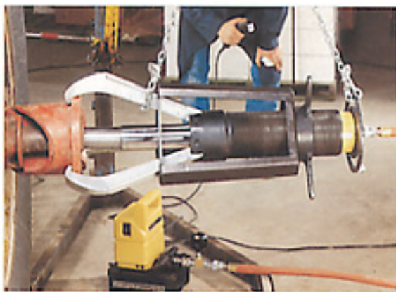
Hub removal from shaft (Model PHB-106)
