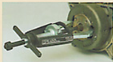
Flywheel removal from snowmobile engine (Model 204)
