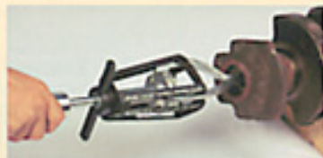
Pilot bearing removal from crankshaft
