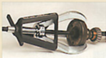
Hub removal from splined shaft (Model 106)
