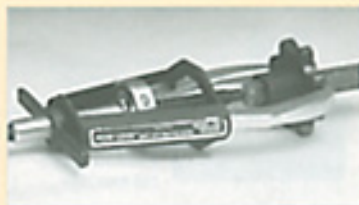
Sprocket removal from shaft (Model 208)
