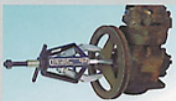
Compressor pulley removal (Model 106)
