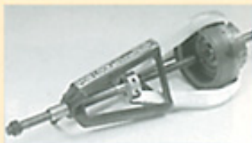
Shaft removal from automatic transmission clutch housing (Model 110)
