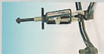
Steering linkage removal (Model 204)
