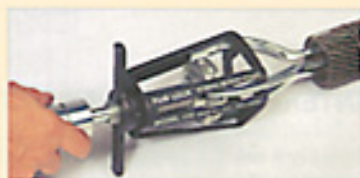
Bushing removal from transmission gear
