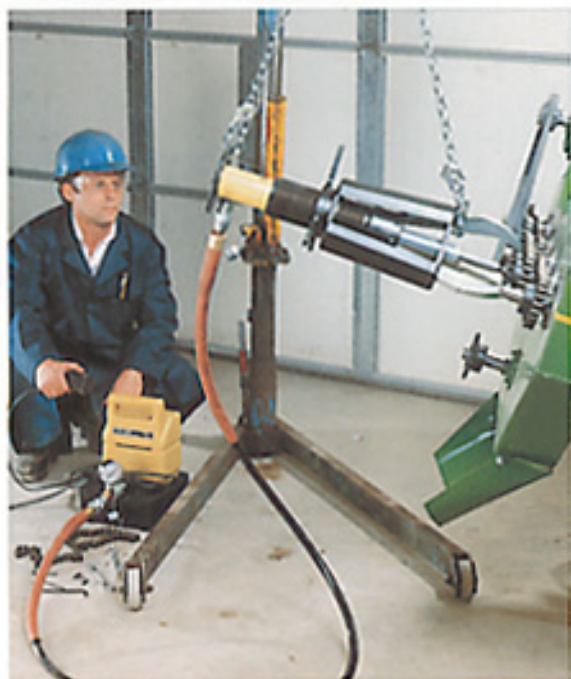
Maximize safety by putting distance between the technician and the application with use of the 10' remote switch.
