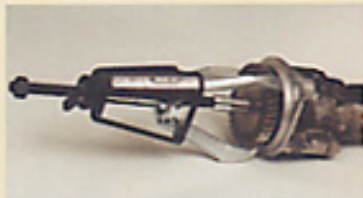
Gear removal from pump (Model 104)
