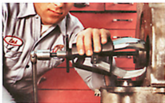
Ball bearing removal (Model 106)
